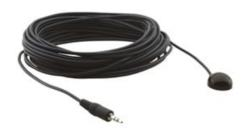
C-A35M/IRRN is a professional IR receiver cable designed for devices that have a 3.5mm external IR receiver port. C-A35M/IRRN enables sending 38kHz IR signals to the device for controlling the device or for routing the IR signal over an extension line
